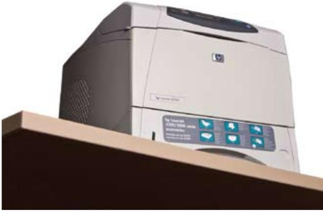
that the DC controller continues trying to heat it instead of flagging an error. In any event, the solution is to replace the fuser.
