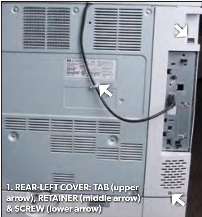
1. REAR-LEFT COVER: TAB (upper arrow), RETAINER (middle arrow) & SCREW (lower arrow)
