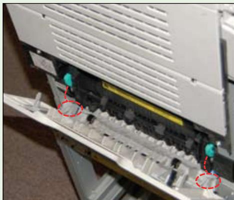
Tabs and levers, all in correct, upright positions. If the jam release levers are left down after pulling out paper, the circled tabs push up them back up, unless the tabs are collapsed. In that case, the lowered levers will result in a startup jam, a very common and confusing error.
