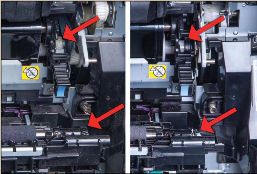
*Look, ma, no gears: top arrows, transfer belt; lower arrows, transfer roller*
