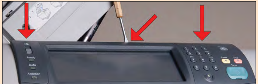
C3 PRY OUT CONTROL PANEL
