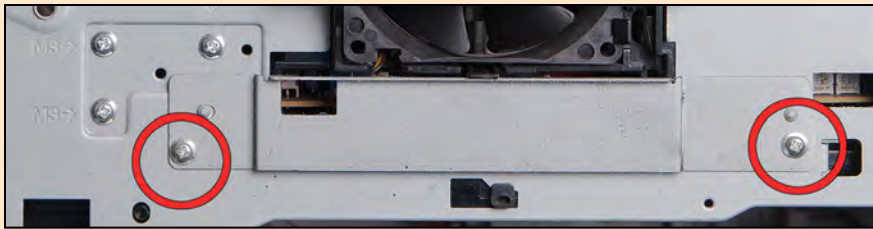
C9 POWER SUPPLY SHIELD
